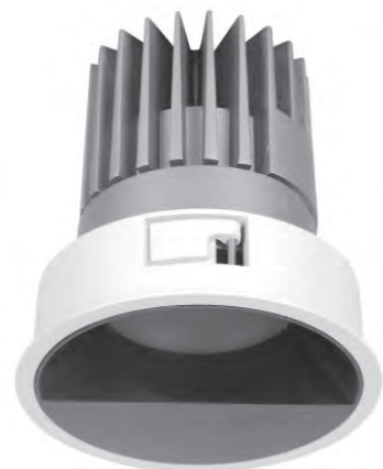
LDB 5A Trim + body: Die-cast aluminium Housing: 1.2mm matt black paint Optic: High efficient reflector
